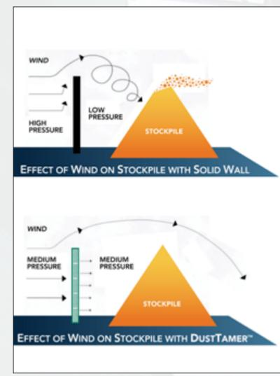
Used as a stand-alone system or in conjunction with fogging, DustTamer provides protection to material stockpiles, truck, rail or loader dump pockets, conveyor transfer points, stacker conveyors and load out silos.
